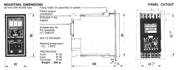
Componibile modular assembly on control panel or 19" rack frames – Panel cutout  $92^{+0.8}\,X_{\rm p}48\,X\,N^{o}-4$
